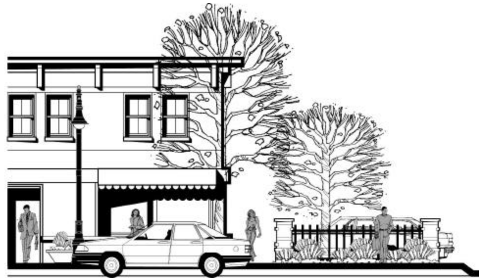
Continuity of form along the block-face is key to the Troost Avenue Action Plan Concept. This is accomplished through continuous building facades or extending the facade-line through features that define and screen surface parking lots next to buildings.
