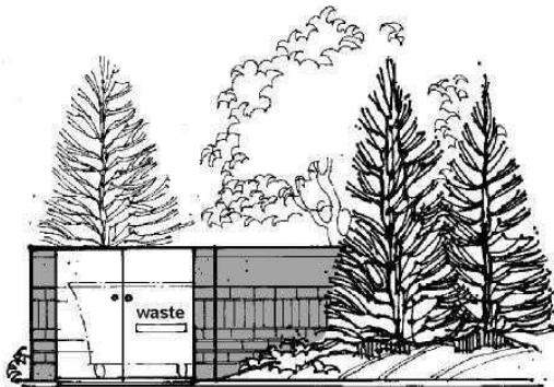
Screening of service equipment and areas should be integrated as part of the building or site.
